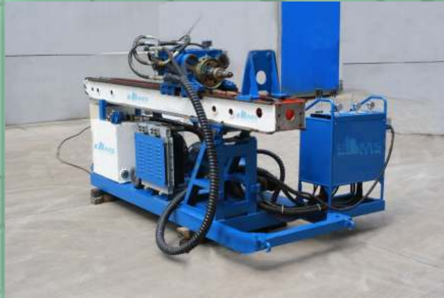
Jet Grout Machine
