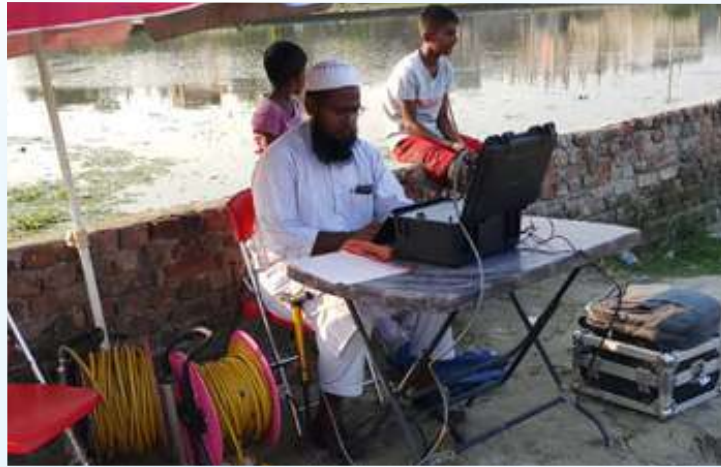
Downhole Seismic Test ASTM D7400
